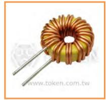
constructed solenoid coils. This is due largely to the smaller number of turns required when the core provides a closed magnetic path. The magnetic flux in a toroid is largely confined to the core, preventing its energy from being absorbed by nearby objects, making toroidal cores essentially self-shielding. The (TCTC) series is suitable for a broad range of applications, such as high-frequency coils and transformers.
