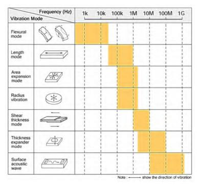
Ceramic Resonator Vibration Mode (Flexural mode, Length mode, Area expansion mode, Radius vibration, Shear thickness mode, Thickness expander mode, Surface acoustic wave) and Frequency Range
